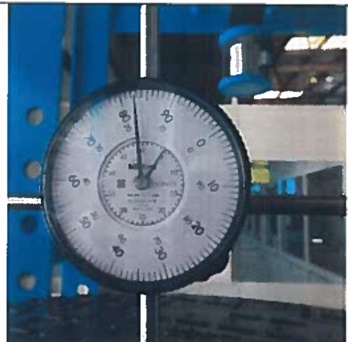
VERIFIED DEFLECTION FINAL READING
