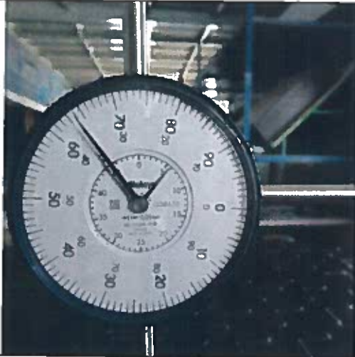
VERIFIED DEFLECTION INITIAL READING
