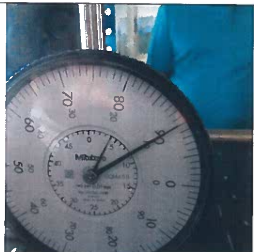
VERIFIED DEFLECTION FINAL READING
