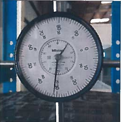
VERIFIED DEFLECTION FINAL READING
