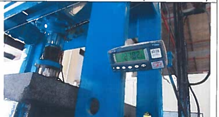
VERIFIED LOAD TEST READING (1200 x 1000 mm)
