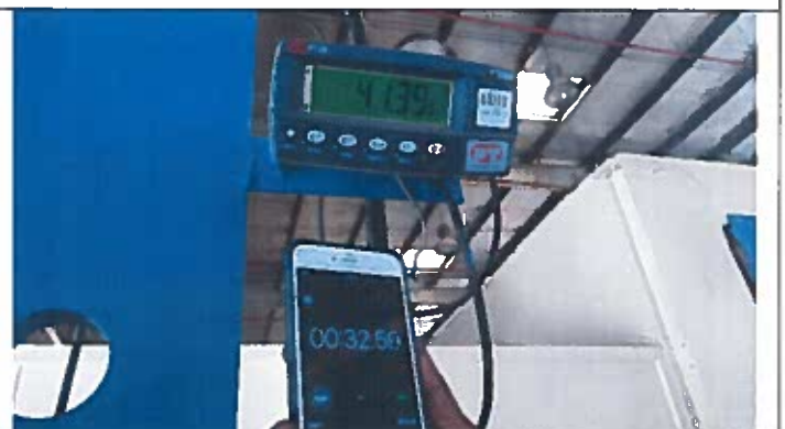
VERIFIED LOAD TEST READING (1200 x 1000 MM)
