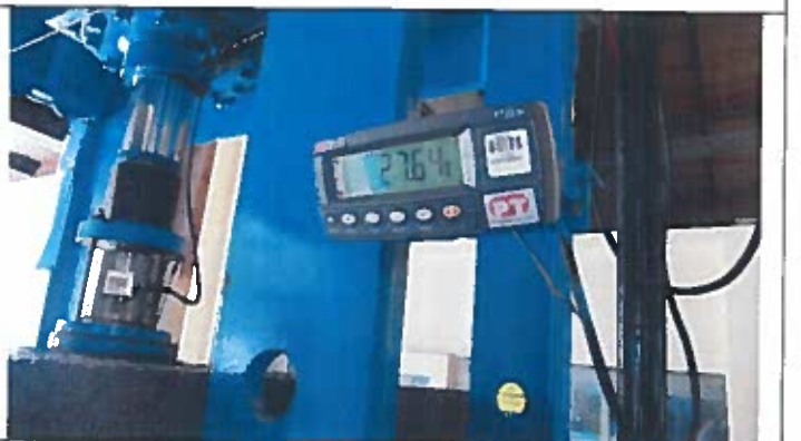
VERIFIED LOAD TEST SECOND READING (1200 x 1000 MM)
