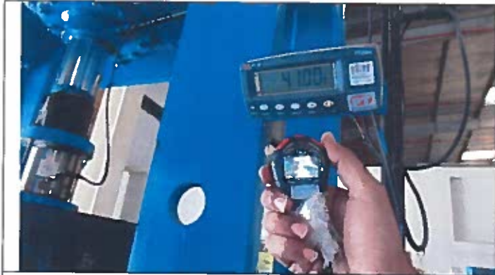
VERIFIED LOAD TEST READING (DN-1000 mm)
