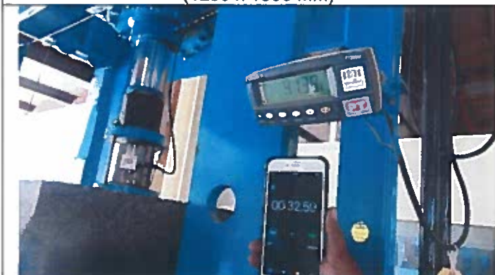
VERIFIED LOAD TEST READING (1200 x 1000 MM)
