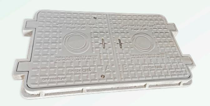
TETRON B1160i Product code TETRON B9060i Available classes : B125 1100 x 600 Clear opening (mm) 900 x 600 Number of covers : 2 Frame height : 70 Hinges (optional) : YES Locking (optional) : YES Single seal gasket (optional) : NO : YES Water tight sealing plate (optional)
